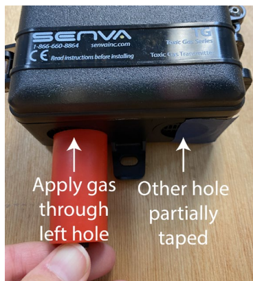
Figure 3: Applying test gas with enclosure closed.
