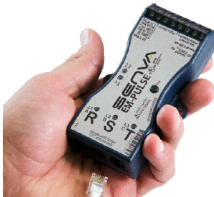
Super compact, low voltage meter base fits in or outside panel. Screw, DIN, and magnetic mounting.
