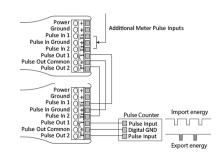
Multi-meter pulse summing. The EMPULSE meter is capable of accepting pulse inputs from one or more meters. The meter will aggregate the pulses and report them as a total sum. The meters must all be set with the same pulse scale.
