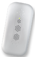
IP54 enclosure (protected from dust and splashing water)
