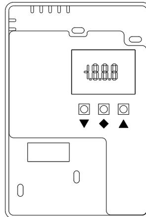
**SPT** Sets the relay turn-on threshold.
