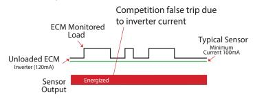
Typical go/no sensors with lower trip points may not change output as they are prone to false trips from the inverter current. The end result is a sensor that cannot distinguish when the ECM is loaded or unloaded.
